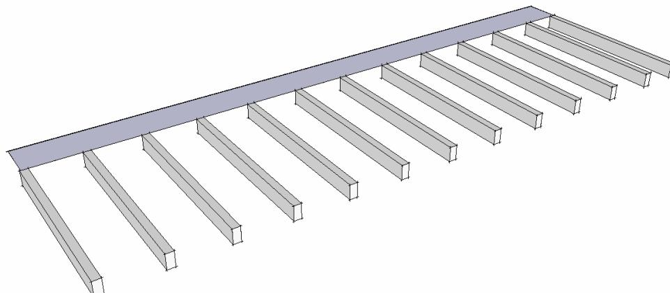
5. So, now let's make a wall trellis. Start with a building and draw a ledger on the wall. (Draw a long rectangle and push-pull it out from the wall a few inches) Then select the top face of the ledger plus 3 edges similar to step 1.
