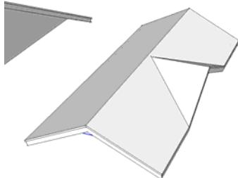
14. Draw a line across the face at a 90 degree angle. This will break the face into 2 faces. Select both faces and 3 edges as shown:
