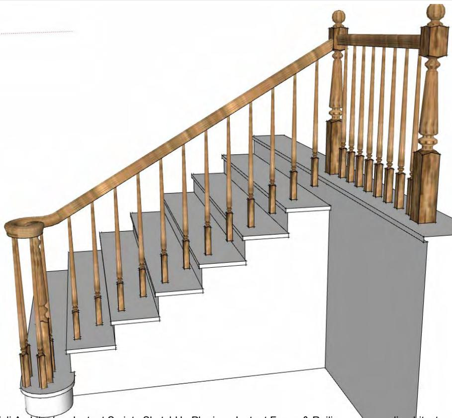
1.6 The spacing is correct but I need do some adjustment. I edit one of the picket components and stretch it down to the tread:
