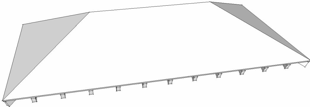
6. Select and erase the 2 groups containing the roof surface and fascia to retain only the beams:
