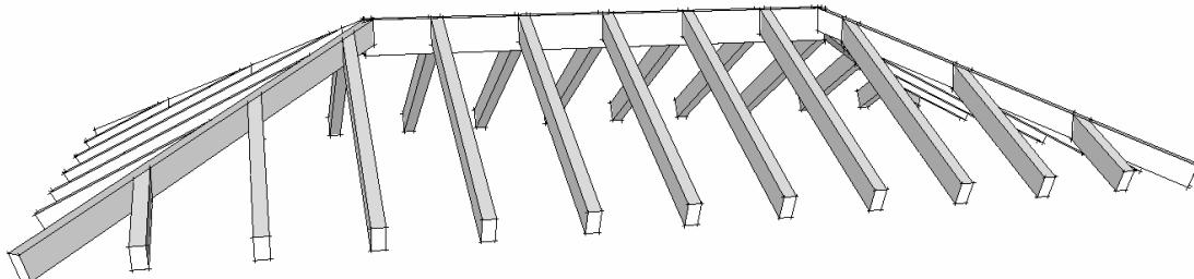
7. Double click the end of a rafter twice to open the end component for editing. Here I draw a horizontal line on the end and used the push-pull tool to make a notch.
