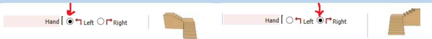
**Flair and Fan Arc stairs** Flair distance is chosen separately for right and left sides for Flair stairs. For Fan Arc stairs the Flair parameter adds a curve in addition to the Flair Angle (see below) and the same for both sides.
