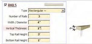
Top Rail Height Measured from "Datum for Infill" setting under "Misc Parameters"
