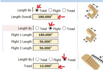
Overall length. Includes all flights. If there is more than one flight, the lengths of the flights will be made equal.
