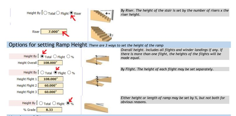
Number of Risers The number of risers can be entered manually for each flight or the script can calculate the number of risers making them less than a maximum riser height. I generally prefer to use maximum riser height.
