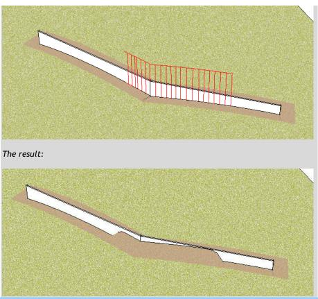
Smooth Terrain Edge Tool Smoothes bumps in the edge of the terrain. It affects edges on one side of the object only. Flatten parameters are similar to the sections above.
