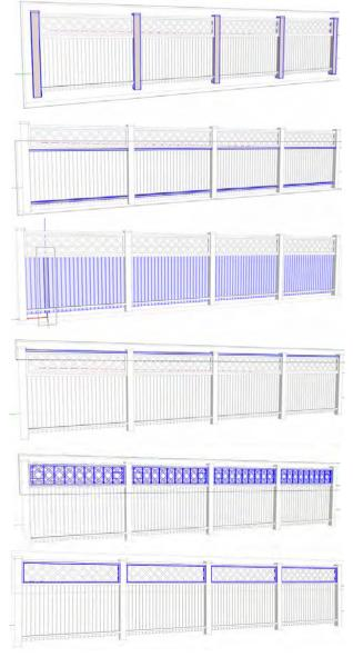
Material Take -Off The script will display a material take off to the screen after each run unless this option is turned off. In addition, an entry is always made into a materials take off list that can be referenced or copy/pasted from at a later time. It is found by selecting "Vali Architects / Instant Fence Railing/ View Take-Off Log"
