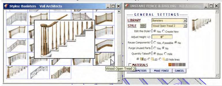
1.4 I want 2 pickets per tread and the tread width is 11" so I retain the preset spacing at 5 1/2". I also retain the Layout parameter at "Ignore Posts" because I do not want the script to re-space the pickets.
