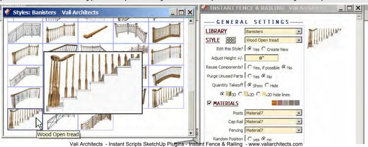
2.2 I don't change the presets because they are set to an 11" tread width. The total of 2 picket thicknesses plus 2 gaps should equal the tread width"
